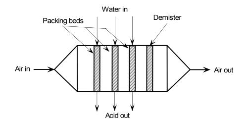
Components of a multi-stage crossflow scrubber Figure 4
