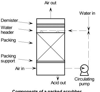
Components of a packed scrubber Figure 1 Figure 1 also shows a couple of disadvantages of packed scrubbers. The main one is that, in order to function properly, the packing needs quite а high water flow rate - about 200 gpm of water for 20.000 cfm of air. Providing this flow as fresh water would be very expensive, and would also produce 200 of slightly gpm effluent. contaminated which would have to be treated. So, instead of using fresh water, most packed scrubbers have
