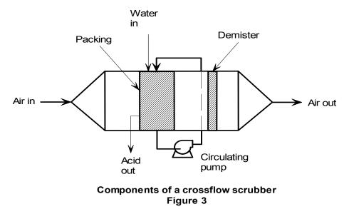
still flows down, a<u>cross</u> the <u>flow</u> of the water. The basic set-up is the same as for conventional packed scrubbers, and a circulating pump is still needed to keep the packing wet.
