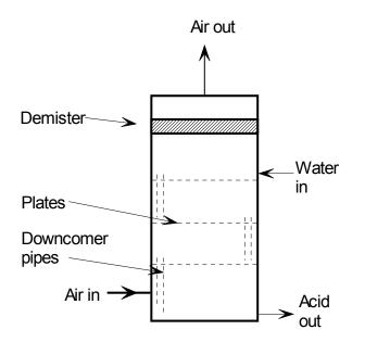
Components of a plate scrubber Figure 2 Because the water forms a pool on each plate, a high flow of water is not needed for efficient contacting - a small flow is needed to flush out dissolved fumes, and also to offset a little weeping that occurs through the holes. due to surface tension effects. In general, recirculation pumps are unnecessary on plate scrubbers. and these scrubbers operate in true countercurrent flow.
